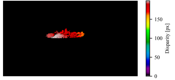
Fig. 7. The resulting filtered disparity image from the wide baseline stereo camera images.
