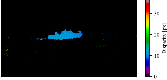
(b) Disparity image after removing points that are far away, compared to fig. 4a. Note some small specks of points remain in the image.
