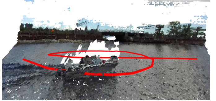
Fig. 1. A point cloud from disparity estimation colored by the rgb image values. The boat in the foreground is visible as well as the quay background. The red line is the estimated track from the complete scenario.
